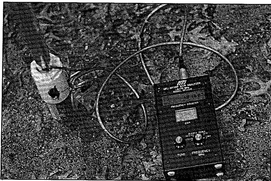
The proof is in the pudding. Here at the base of the 160 meter center loaded vertical you can see the mica capacitor, and at the rear a portion of the RF choke described in the text. You will also note that the resonant frequency is 1.8168 MHz.
