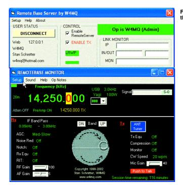
Figure 2—Operation displays used to set up, monitor and control the remote base server.
