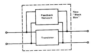
For example, the above combination of transistor and
