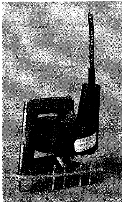
Here is a standard television-flyback transformer. Modifying it by adding a new primary winding is the heart of the Poor Man's Plasma Globe.
