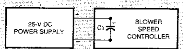
Fig. 6. When you're ready to do preliminary testing of the low-voltage side of the Blower Speed Control, temporarily hook up a 25-volt DC power supply in this way to power the circuit.
