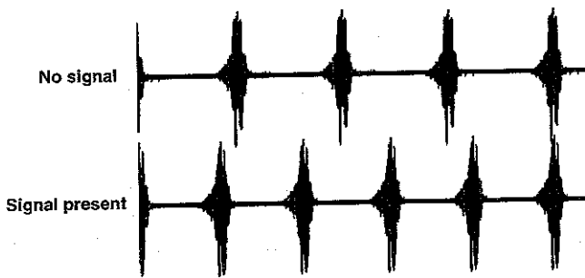
Fig. 4. Bursts of rf in a self-quenching super-regen receiver. The no-signal quench frequency - upper trace - is about 80kHz. The increased pulse rate - with a consequent increase in supply current drawn - is seen in the lower trace. The ragged appearance of the rf pulses is due to sub-sampling of the waveform by the digital storage oscilloscope used.
