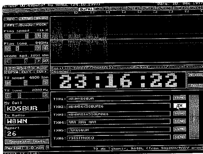
Figure 2— MS DSP , written by Tihomir Heidelberg, 9A4GL, is popular among HSCW operators. Above the digital clock is the main receive buffer. When a burst is heard, the operator marks the buffer spot and saves the burst to one of eight buffers above. During the next transmit period the saved buffer areas are replayed while varying the speed and tone with controls to the left. Transmit data is changed (lower left) and selected as necessary (lower right).
