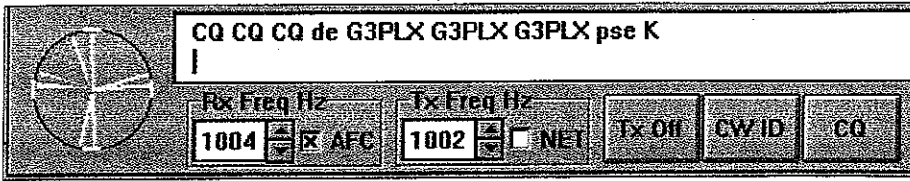
Screenshot of the control panel of the PSK31 Windows program, with the tuning display showing a slightly noisy QPSK signal, and showing the fine-tuning controls of the receive and transmit audio tones.
