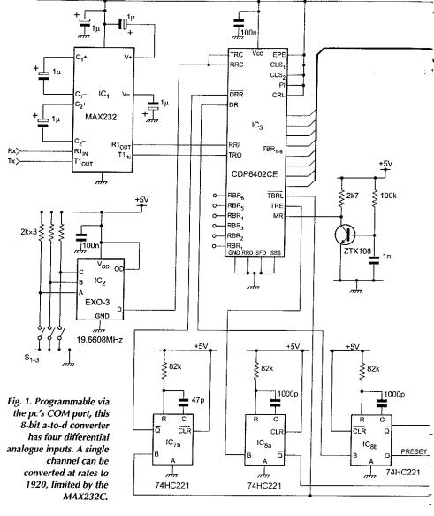
the command is received from the computer. The data received status line DR goes high, and edge-triggered monostable IC8b provides a low level pulse of about  $82\mu s$  duration to the WRITE input of the a-to-d.
