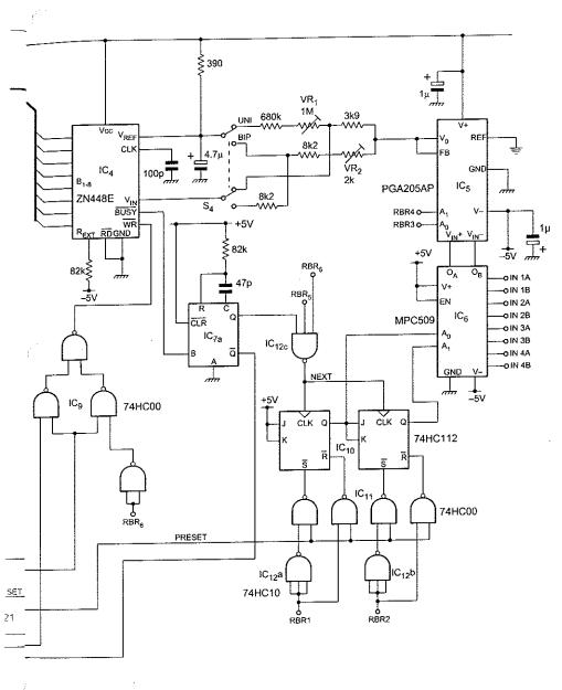
from DR, but then from the transmitter register empty, TRE, status flag of the uart. This signals that the last conversion has been sent to the computer, and that the UART is ready for new data. Again, the pulse is about 82µs duration.
